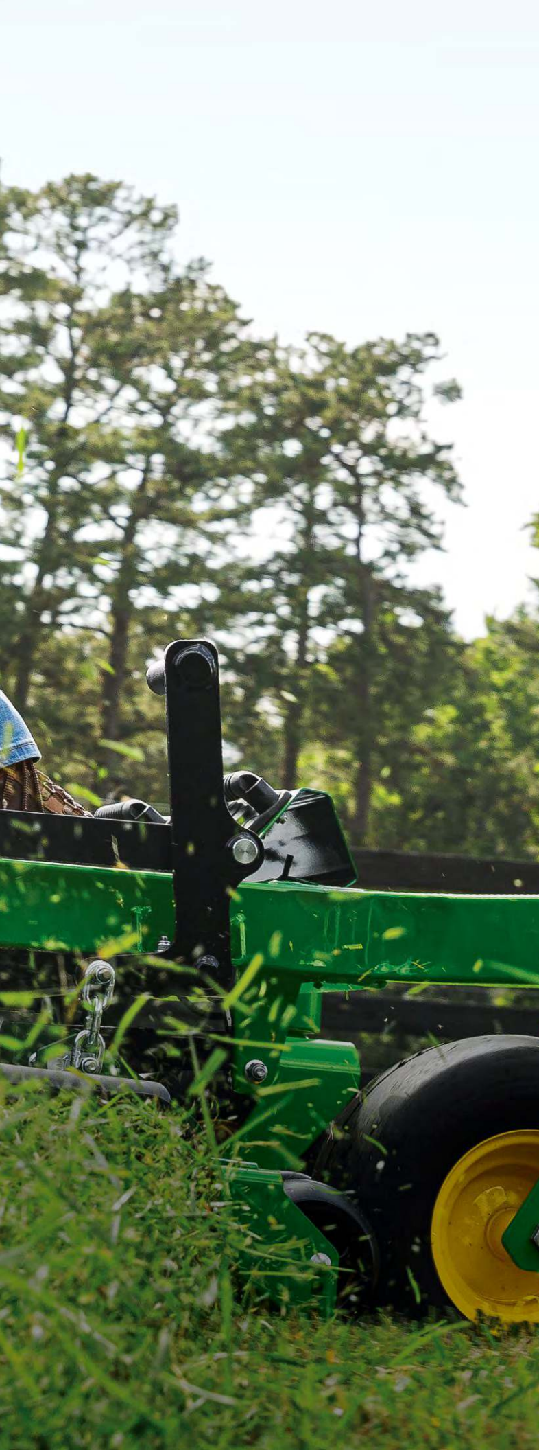
Z700's High-Capacity PRO Mower Deck. Designed for large properties and tough mowing conditions, these heavy-duty mowers are forged from thick 9-gauge steel. Available in 48-, 54- and 60-in with commercial grade reinforcements.
