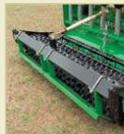
Optional scraper bar for clay or wet conditions
