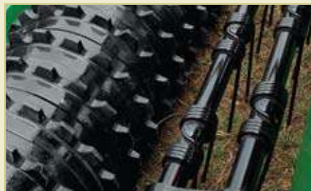
Fiberglass ring corrugated roller ensures seed-to-soil contact
