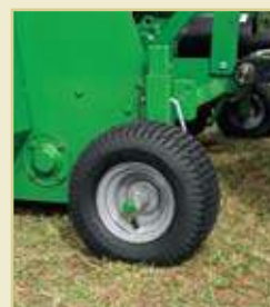
Optional front gauge wheels (cannot be used with optional front gauge roller)
