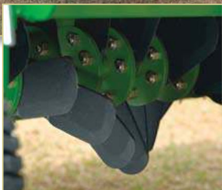
Straight blade aerator rotor aerates and incorporates seed
