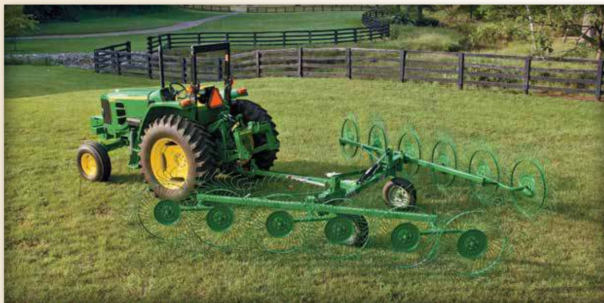
The WR30 Series Carted Wheel Rakes feature 15 to 24 foot raking widths for gentle, efficient windrowing. Each model folds 9-feet 6-inches wide or less for easy transporting and convenient storage.
