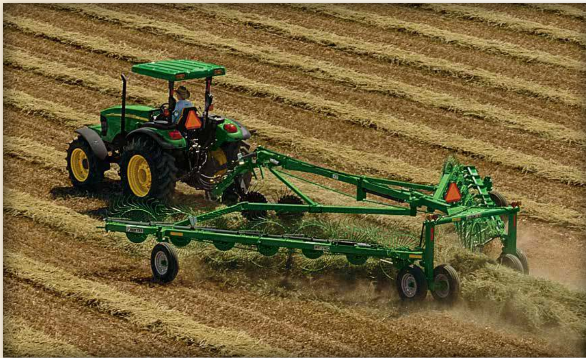
Frontier High-Capacity Wheel Rakes effectively handle heavy crops on rough terrain. Choose models with 12, 14, or 16 wheels.
