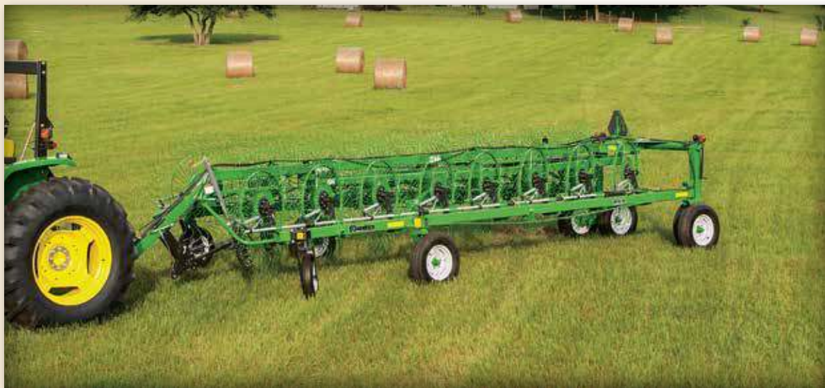
Frontier High-Capacity Rakes open and close hydraulically. Transport widths are 8 feet (2.4 m), making it easy to negotiate narrow roads and gates. Transport lights are standard on WR1214 and WR1216.
