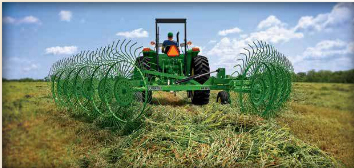
The WR30 Series comes in 8-, 10-, or 12-wheel options. With 55-inch wheel diameters and 40 rugged, steel tines per wheel, you get fluffier, more-even windrows for better quality bales.
